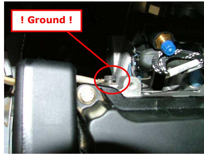
**POWER STEERING ECU LOCATION / FIXATION (For optional racing loom)**
