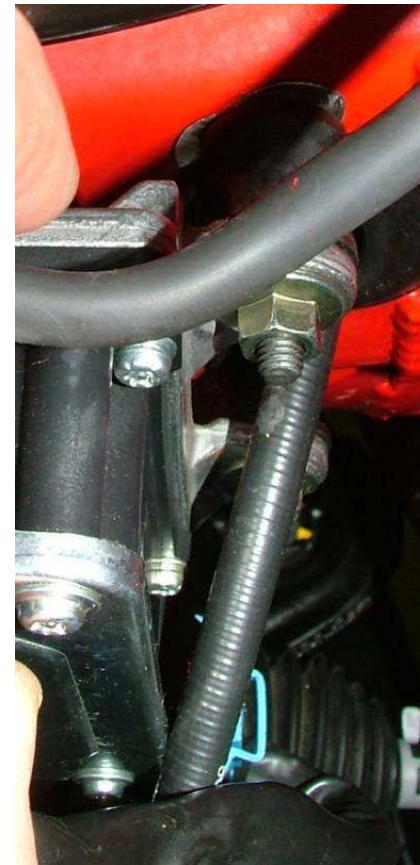
**NOTA :** Fit the power steering ECU with connectors turned in bottom way. This way, if brake fluid tank is leaking, the fluid will not fall on connectors.
